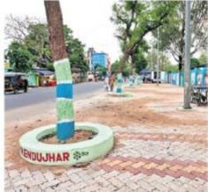
tion works and renovation of ponds in various wards of Keonjhar town are being undertaken for the last two years where paver blocks are used. The paver blocks get heated during the daytime and radiate the heat during night.
