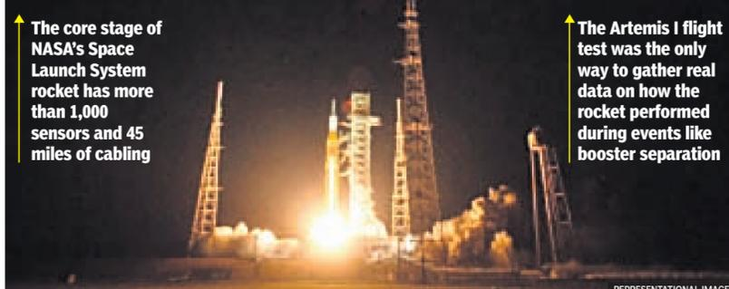
The core stage of NASA's Space Launch System rocket has more than 1,000 sensors and 45 miles of cabling
