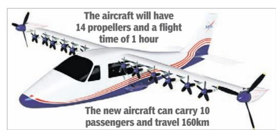
The aircraft will have 14 propellers and a flight time of 1 hour
